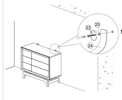
5. Finally, attach safety strap (24) and washer (25) using 4x30mm screw (23) to the wall.
