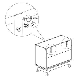
4. Add safety strap (24), washer (25) using 3.5x15mm screw (21) to back of cabinet.
